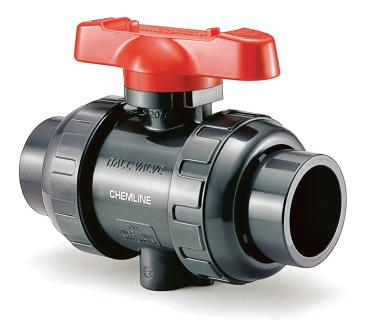
The Chemline Type 21 True Union Ball valve incorporates state of the art features for long term performance. This is a full port, full blocking True Union valve pressure rated at 16 bar (230 psi)4. Double stem o-rings and Safety Shear stem design provide for a high degree of safety on hazardous fluid applications. All sizes have an ISO standard actuator mounting platform integral to the valve body. This provides for sturdy and secure mounting of pneumatic or electric actuators.
