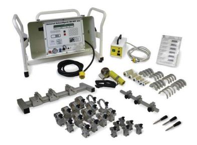
The **High Performance Fusion** is a welding machine for the beadless electro-socket welding of pipes and fittings from OD 20 to 110 mm (1/2" to 4") for PP and OD 20 to 63 mm (1/2" to 2") for PVDF in the workshop or in the field. The device is composed of the welding machine with entry pad and display, protective tube frame, welding and power supply cables, inflatable balloon, barcode reading pen and serial authorization card.
