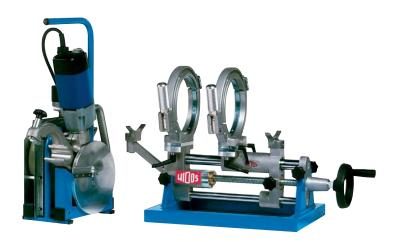
The **Maxiplast** is a welding machine for heating element butt welding PE, PP, PVDF and ECTFE pipes and fittings from OD 50 to OD 160 mm (1-1/2" to 6") in the workshop or in the field. It has two large aluminum pipe clamps which accept reducers for different pipe sizes, as well as two narrow fitting clamps for fittings with short legs. The clamps also swivel up to 15° on each side for the fabrication of segmented bends.
