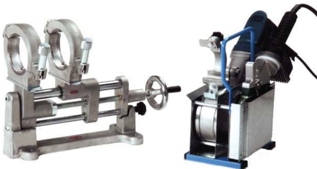
Welder and Pipe Clamps
