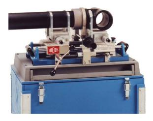
The \$3500 bench socket fusion tool is ideal for socket fusion of larger diameter pipe and fittings. It is capable of socket welding PE, PP and PVDF pipes and fittings from OD 20mm to OD 110mm (1/2" to 4") in the workshop or in the field. Special angled clamps simplify pipe and fittings clamping. A simplified process means little change out is required when switching sizes. Mechanical stops automatically set the socket depth for a perfect weld every time.
