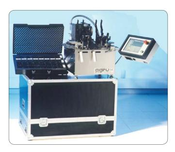
The **SP110** is an automatic welding machine for heating element infrared welding of PE, PP, PVDF and ECTFE pipes and fittings from OD 20 to OD 110 mm (1/2" to 4") in the workshop or in the field. It has two large aluminum pipe clamps which accept reducers for different pipe sizes, as well as two narrow fitting clamps for fittings with short legs.
