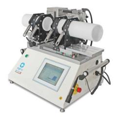
The **SP110S.10S** is an automatic welding machine for heating element infrared welding of PE, PP, PVDF, ECTFE and PFA pipes and fittings from OD 20 to OD 110 mm and 1/2" to 2" IPS sizes. in the workshop or in the field. It has two large aluminum pipe clamps which accept reducers for different pipe sizes, as well as two narrow fitting clamps for fittings with short legs.
